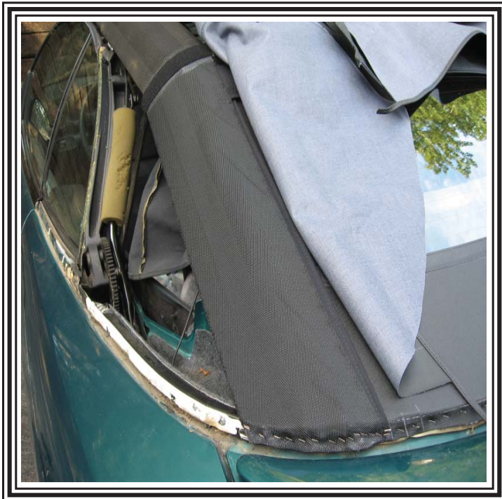
Staple the rear quarter pads to the trim stick.
