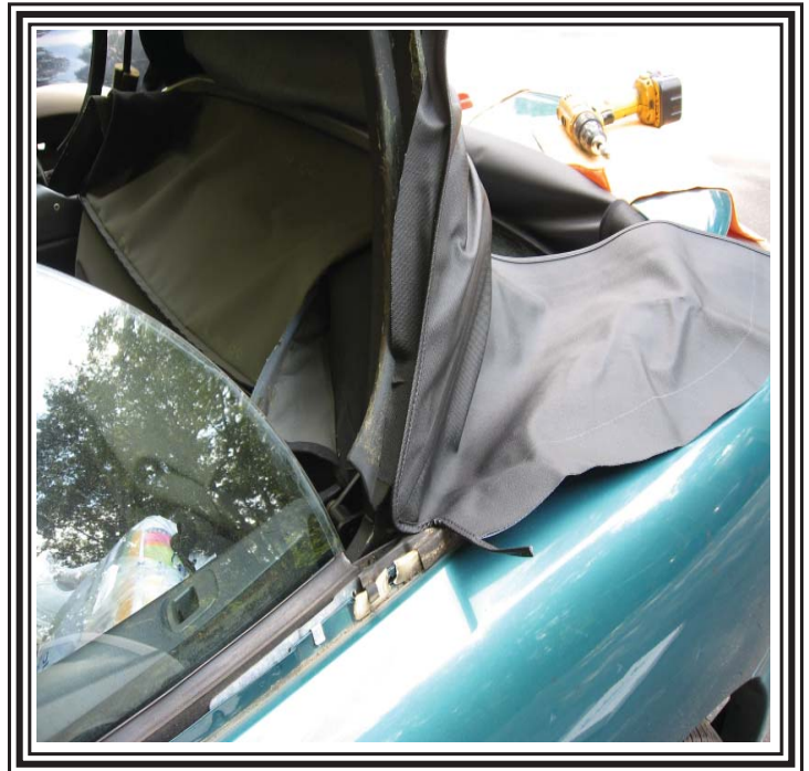
Slide the pocket of the corner of the top over the end of the frame. This will lock in the corner at the bottom of the quarter.
