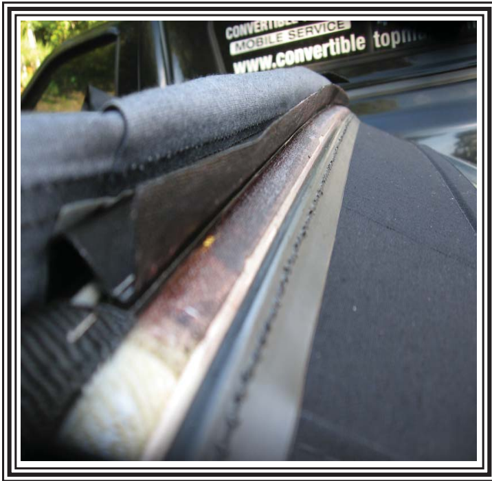
Glue the back remainder of the bow listing to the rear bow.
