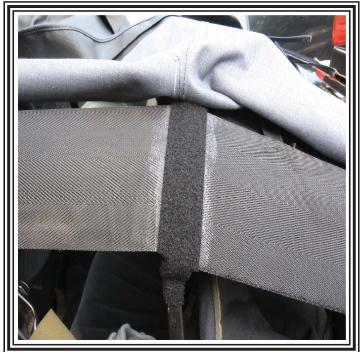
Use a piece of 2" self adhesive velcro pile to pad out the rear bow area.
