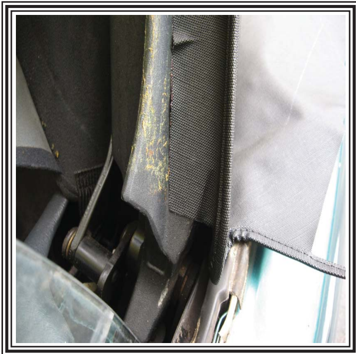
This is a picture of the gluing and locked in channel flap.
