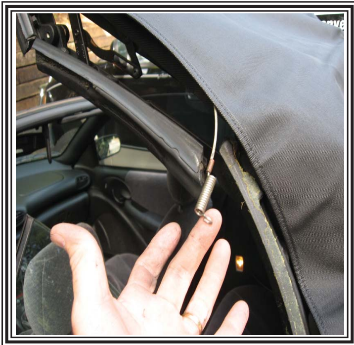
Run the side cables through the wire sleeves of the top on both the passenger and drivers side of the top.
