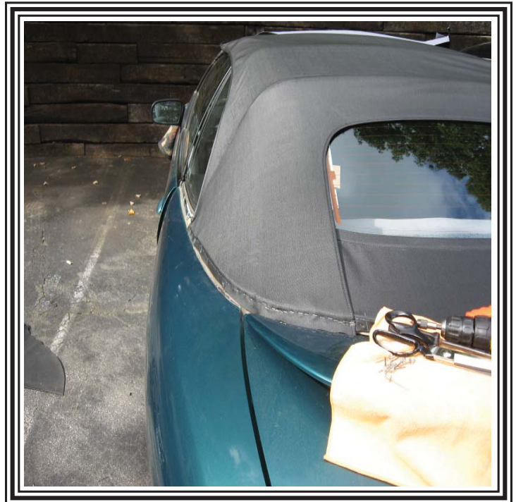
Staple the rear quarters to the rear tacking strip.
