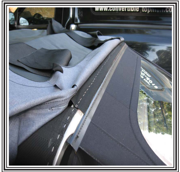
This a view of the rear bow listing stapled and glued down.
