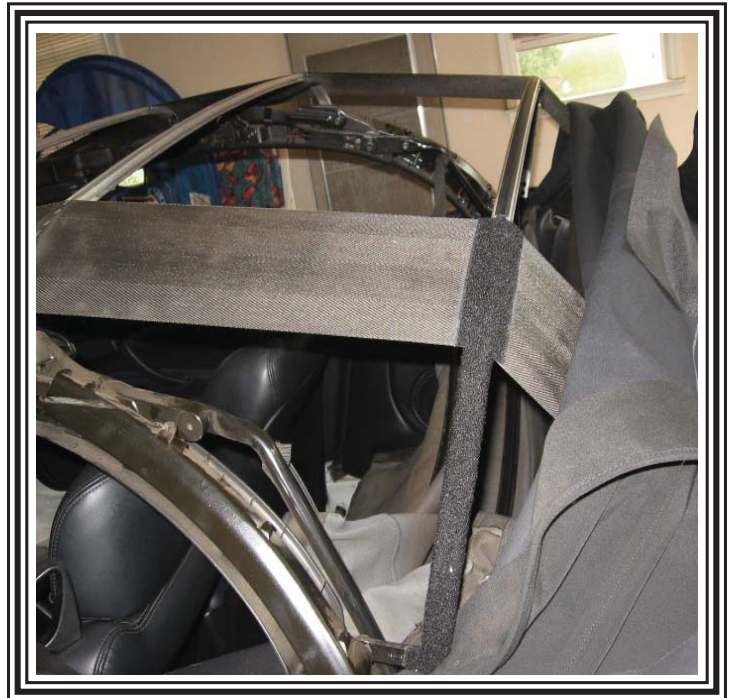
Pad out the rear bow on the corners using self sticking velcro pile. It helps protect the top and looks better.
