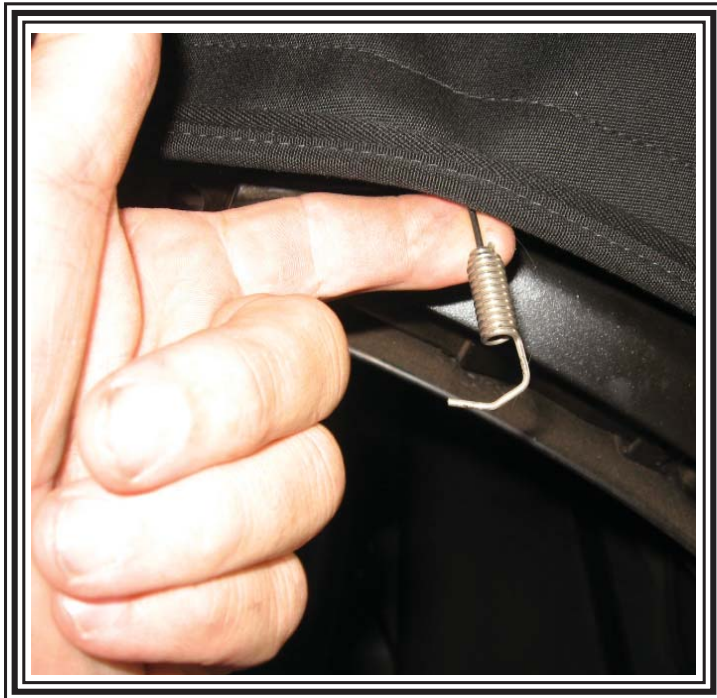
This is a closer look at the cable end coming out underneath the top.
