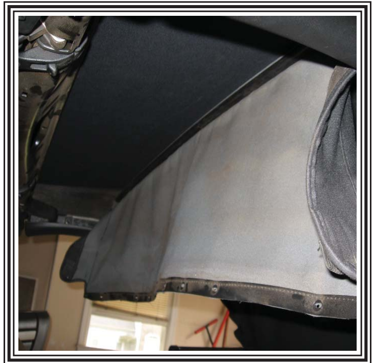
Latch the front header bow, glue all three bow listings and fasten up the headliner.
