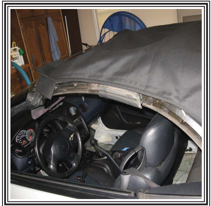
Thread the cable through the wire sleeve on the edge of the top on both sides. In this view the cable is already through.
