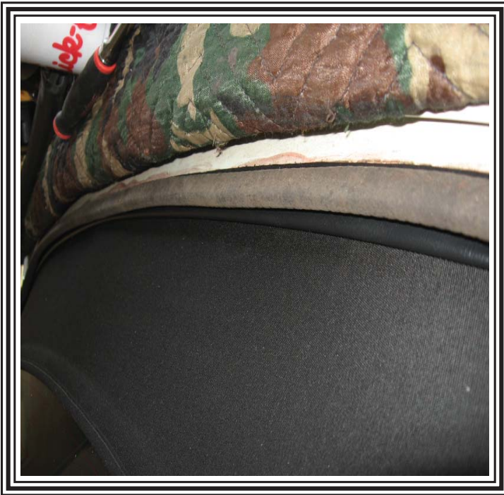
Snap on the windlace and push it up to the body of the car.
