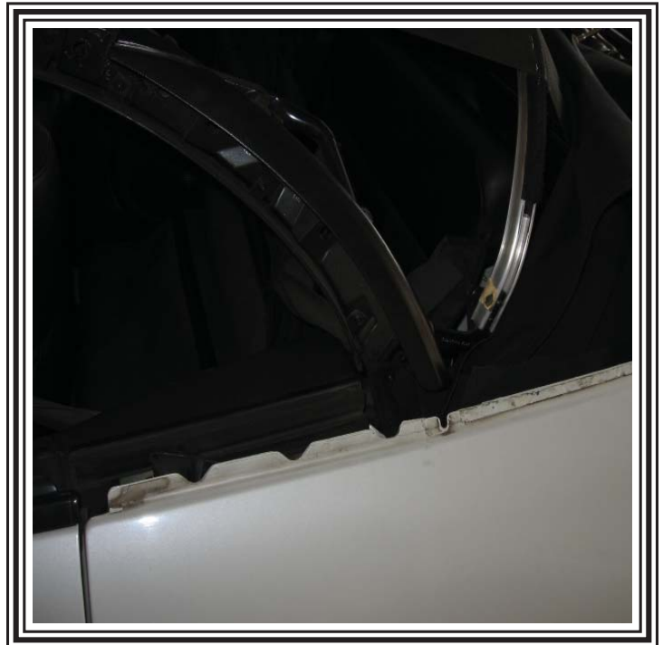
You then can reinstall the rear trim stick.
