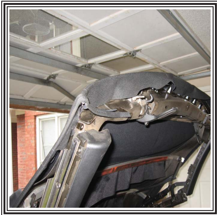
Glue the front of the top on each side.
