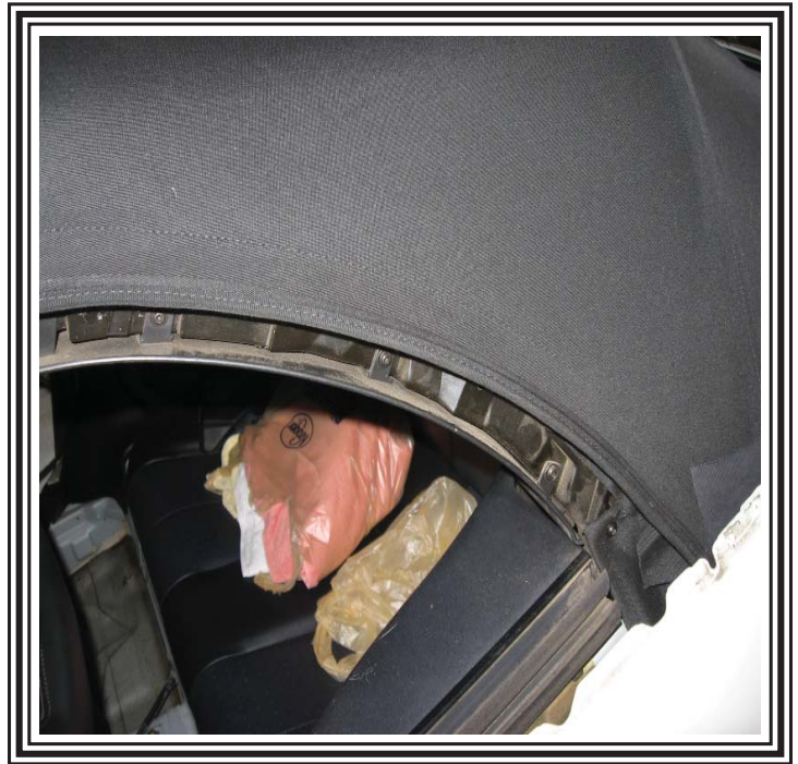
Glue and re-attach the rear quarter channel flaps back by the quarter glass window channel (also known as the C-pillar post on most cars).
