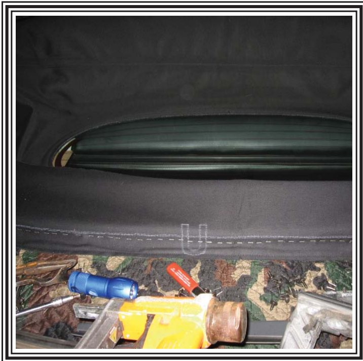
Staple the center of the top to the trim stick making sure the line is at the top of the trim stick, then work your way around each side.
