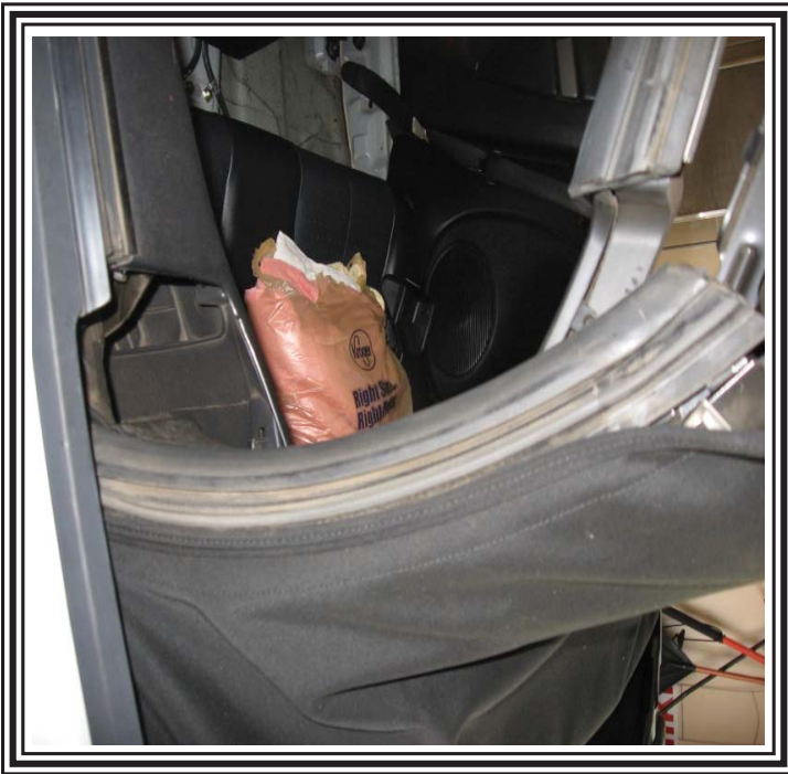
Re-install all the weather stripping.
