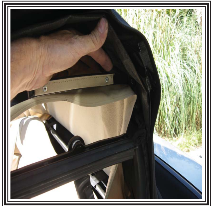
Do the same on the other side of the top by pop-riveting the vinyl strap to side rail of the frame.
