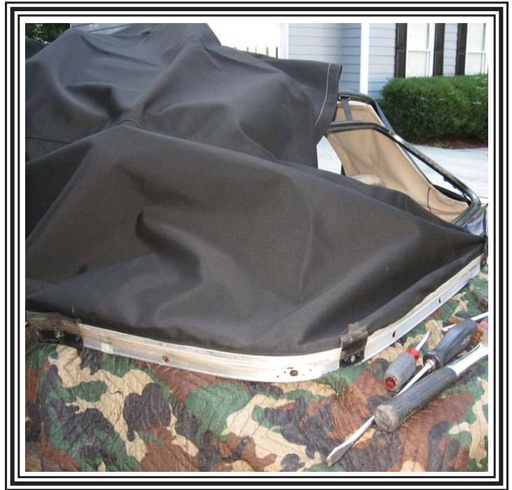
This is another view of the top pulled half way around the awning rail trim stick.
