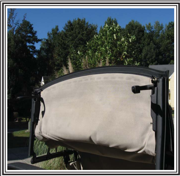
This picture shows the completed installation of the top and the front header bow.
