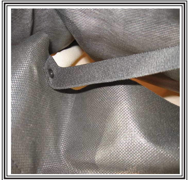
Position the elastic strap at the center of the top. Pop-rivet the strap to bow between top and headliner like in the picture above.
