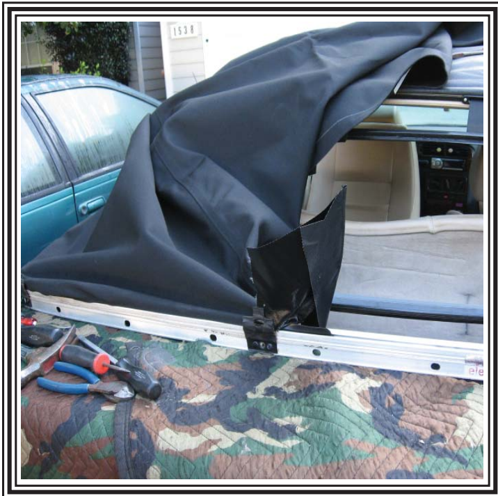
This picture shows the top almost fully pulled around the awning rail trim stick.
