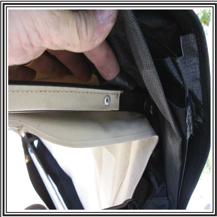
Pop-rivet the herculite vinyl strap to the side-rail of frame of the top like the picture above.
