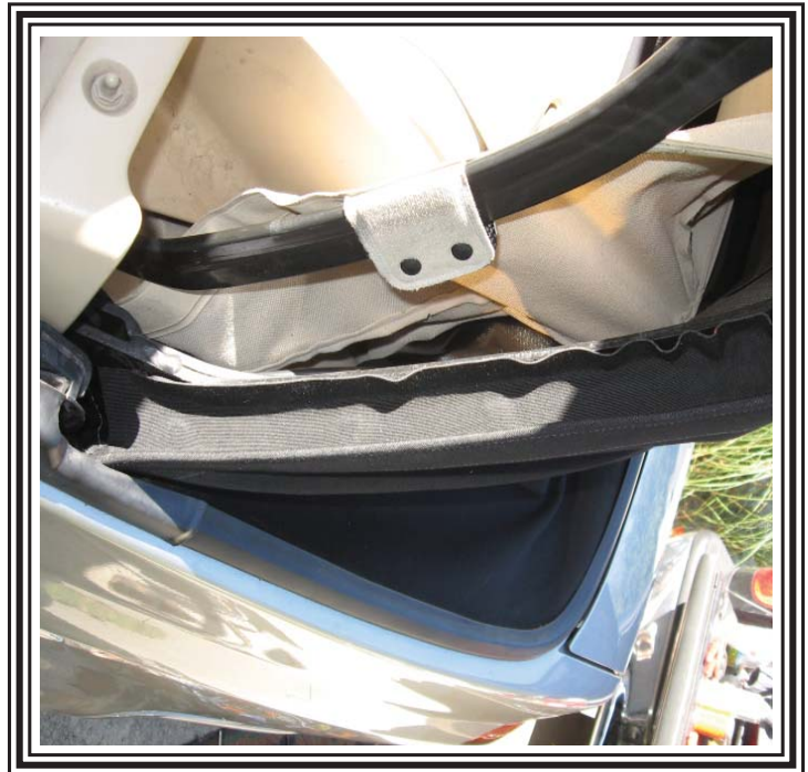
Lay out the top's quarter channel flaps and cement them to the C pillar post as shown above in this picture.
