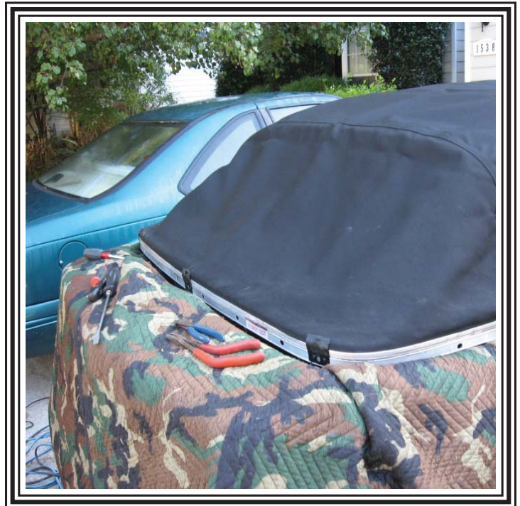
This is a view of the rear of the top after the top has been fully pulled around the rear of the trim stick.
