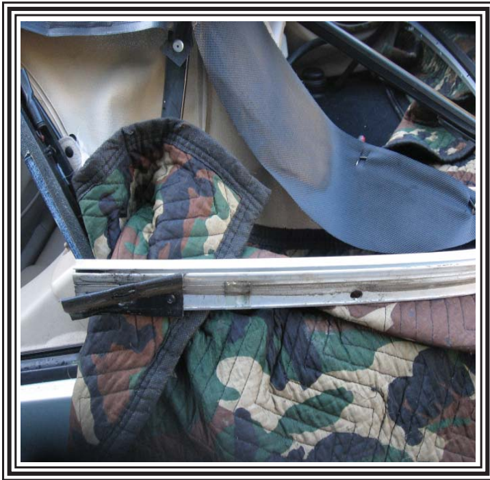
These pictures show how to slide top into the awning rail trim stick. Starting from the drivers side working your way to the passenger side.
