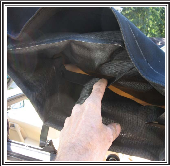
This is pointing out the elastic strap that is on both sides of the car.
